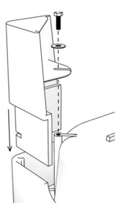
Secure with a supplied washer and hex bolt, using the 10mm wrench. Repeat for the other 3 legs.
