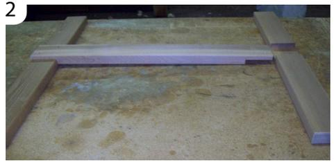
3 Apply wood glue in the cut out sections of the legs. Insert the cross piece into cut outs on the 2x4 legs and attach the cross piece using 1 1/4" screws. Repeat for other leg section.
